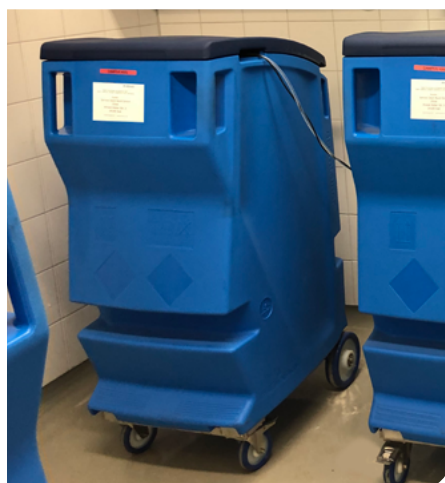
Fig. 3: Drum containers allow the chemical drums to be moved easily and double as leakage protection.
