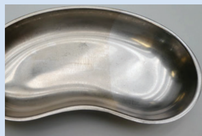
Figure 3: Kidney dish before basic cleaning (left) and after partial basic cleaning with neodisher® IR in an immersion bath (right)
