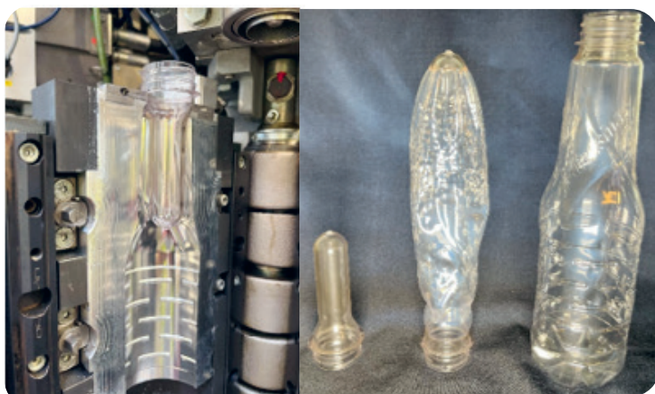
The evolution of the juice bottle: From preform to designer bottle
