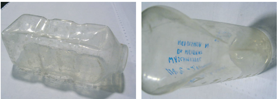
Fig. 9-5: View of drinking bottles with deformations
