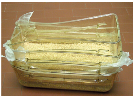
Fig. 9-6: Deformation of cage bases on the left, cracks in cage shells on the right
