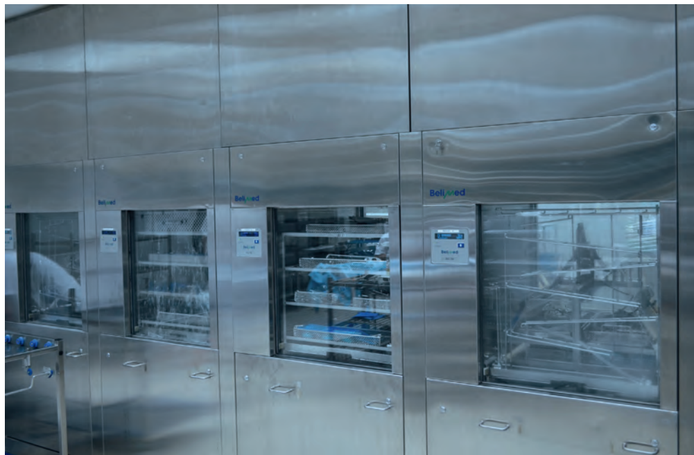
Fig. 1: Processing of medical devices using the mildly alkaline enzymatic cleaner neodisher® MediClean forte in washer disinfectors at the Marienhospital Gelsenkirchen.
